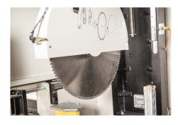
The cutting unit with a 550 mm diameter saw blade for cutting at every angle between 30° and 150° offers a wide cutting range to users.
