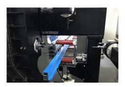
Four air-cooled spindles which are positioned and can process in different angles provide easy and unlimited operation on 4 surfaces of the profile. When upper spindle can be positioned at every angle between  $0^{\circ}-45^{\circ}$ , frontal spindle can be positioned at every angle between  $45^{\circ}-135^{\circ}$ .
